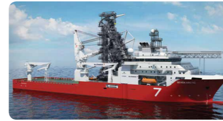
The Seven Arctic benefits from a 900t offshore crane
